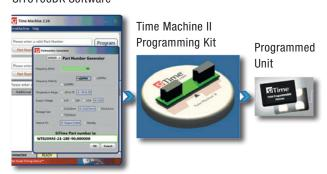
The starter kit includes three adapter cards for the reception of the 6 possible MEMS oscillator housing types, as well as some samples of field-programmable oscillators. Via the supplied USB cable, the Time Machine  $\rm II^{TM}$  can connect to a computer. The Windows compatible software is available by included USB Flash Drive or can be downloaded from SiTime Website.
