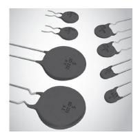
**Semitec's Power Thermistor D2 series**, are negative temperature coefficient (NTC) thermistors, which can be used to suppress inrush currents of electric circuits, when added in series with the circuit which has to be protected.
