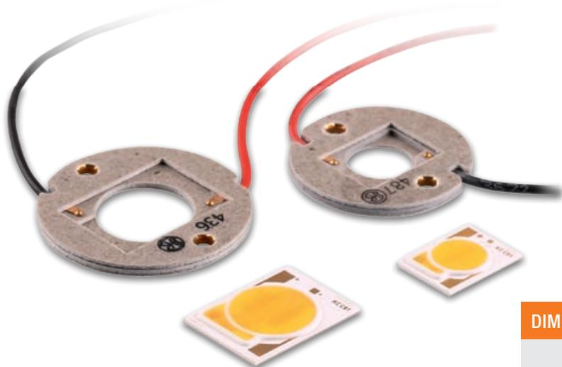
**Citizen Electronics** has developed the Dim-to-Warm COB series CLCOx0 which can change the colour temperature from 2700 K to 1800 K and 3150 K to 1850 K by dimming with a triac dimmer or potentiometer. The aim of this product is to imitate the effect of the incandescent lamp which became warmer by dimming. Those COBs can be used in combination with solderfree holders from Bender+Wirth, which we also available from Endrich stock.
