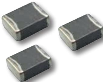
**ABC's DP Series are inductors in chip size.** Externally they look like chip ferrite beads or multilayer chip inductors. The internal construction however, consists of an enamelled flat copper wire wound in  $\alpha$  style which helps to reduce the DC losses (DCR) to a minimum. The core material consists of a partly amorphous metal alloy powder which helps to reduce the AC losses (core loss) to a minimum.
