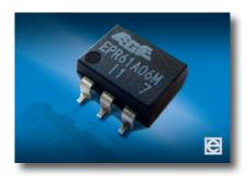
The **EPR311A066107EZ MOSFET Relay** from Excel Cell (ECE) is specifically designed for high current applications (continuous: 2.5 A, peak: 4A), commonly found in industrial equipment. The MOSFET relay is a possible solid-state replacement for single-pole, normally-open (Form 1 A) electromechanical relays.
