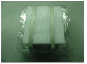
3. Put foam which has 1cm thickness on the top of tray & fix it by package machine.
