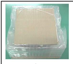
Piled up trays put in a bag and vacuum sealed.
