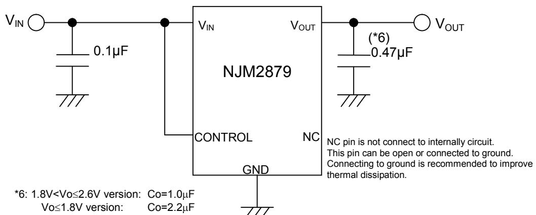
Connect CONTROL Pin to  $V_{IN}$  Pin
