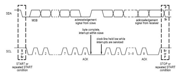
Figure 1-1 I2C Serial Data Transfer Format
