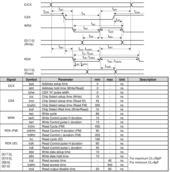
Note: Ta = -30 to 70 ℃, VDDI=1.65V to 3.3V, VCI=2.5V to 3.3V, VSS=0V
