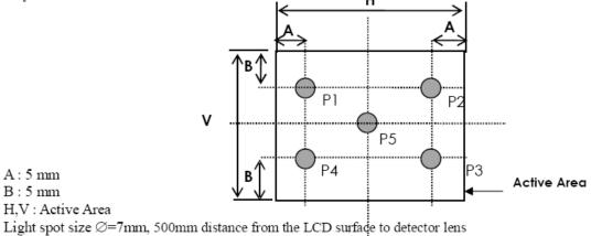
Light spot size O = /mm, 500mm distance from the LCD surface to detector left measurement instrument is TOPCON's luminance meter BM-5
