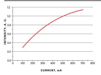
Test Conditions: Case Temperature ( $T_{\rm C}$ )= 20 °C CW operation
