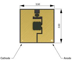
Devices are placed with the cathode to the left so the polarity direction is cathode to anode.
