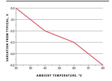
Test Conditions: Forward Voltage ( $I_{\rm F}$ ) = 500 mA CW Operation
