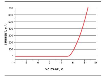
Test Conditions: Ambient Temperature ( $T_A$ ) = 25 °C Electrical sweep from -5 V to 15 V at 700 mA
