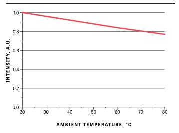
Test Conditions: Forward Voltage  $(I_F) = 500 \text{ mA}$  CW operation
